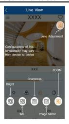
②: Zoom adjustment (this function is only available for cameras with motorized lens).
