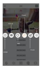
Please control the PTZ by sliding the image in the direction of the arrow marked on the image. The PTZ will automatically focus on the little red circle by tapping on the image. Then the 3D function
